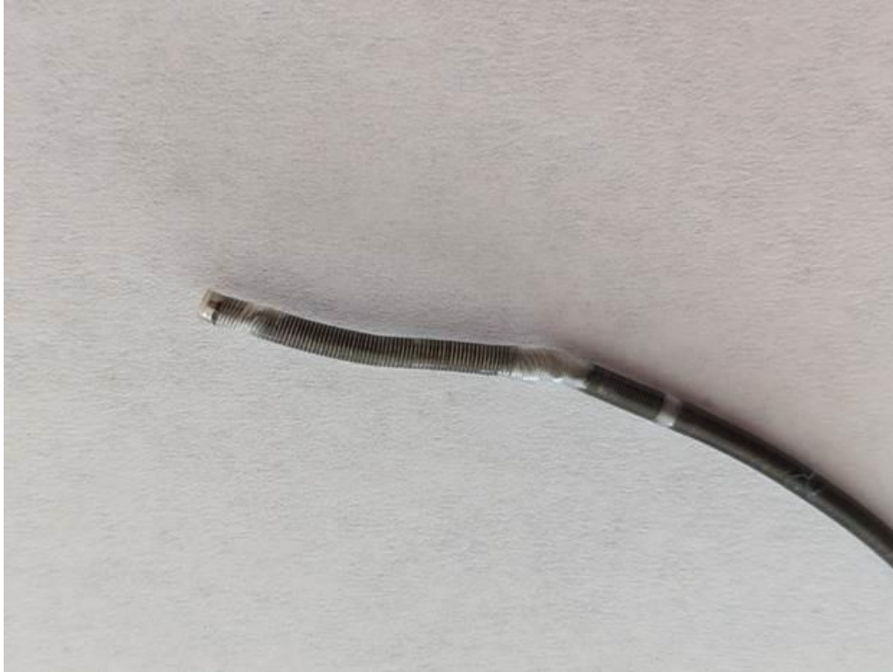
A damaged distal tip of a Jet 7 device
